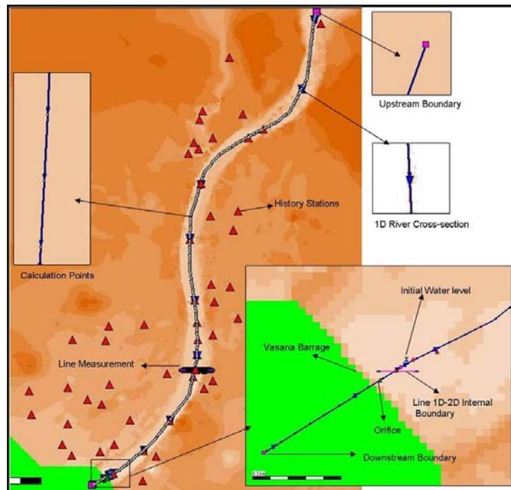
**Figure 8 SOBEK Schematisation in 1D2D with details**
