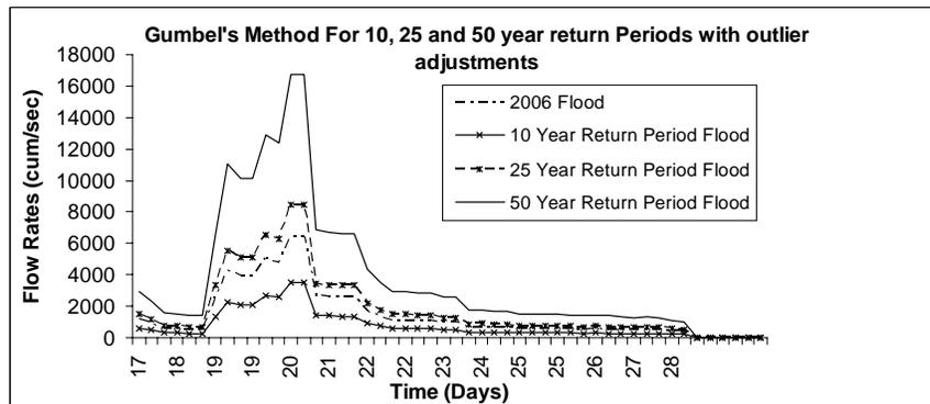
**Figure 6 Gumbel's Method of flood Magnitude – frequency analysis for 10, 25 and 50 years of return period after adjusting the lower outliers**
