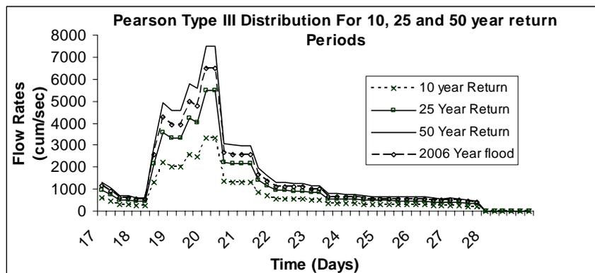
**Figure 7 Log Person Type – III Flood Magnitude – frequency analysis for 10, 25 and 50 years of return period with year 2006 data**
