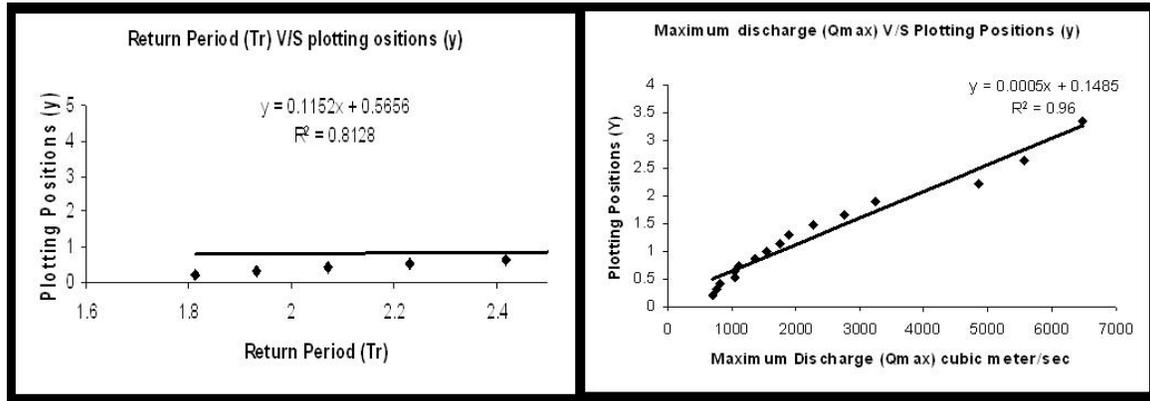
**Figure 5: Gumbel's plots for the probability distribution of return periods after adjusting lower outliers**
