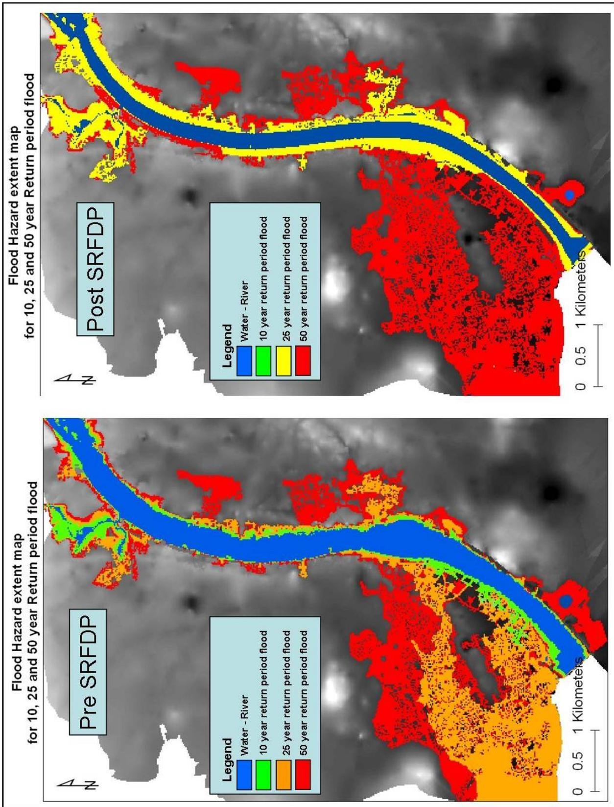
Figure 13 Comparison of Pre and Post SRFDP flood hazard extents
